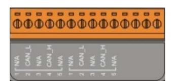
Table 2-2: CAN bus Connector Pin Assignment
