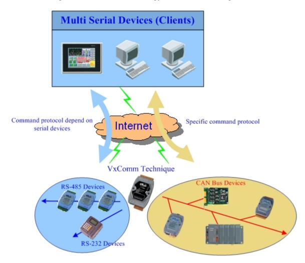
The VxComm technology can be used to simulate COM/CAN ports of the I-7540D to become a COM port of PC. With the help of VxComm driver, users can access the remote COM/CAN ports of the I-7540D just as them would access the PC's COM port.
