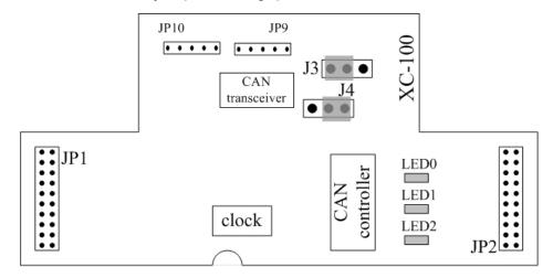
Figure 2-5 XC100 I/O expansion board LAYOUT
