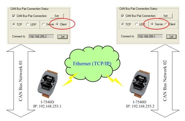
After setting "CAN Bus Pair connection Status" of the two I-7540D and re-start the system of them, CAN messages between CAN Network 01 and CAN Network 02 can be exchanged by TCP/IP protocol through Ethernet network.
