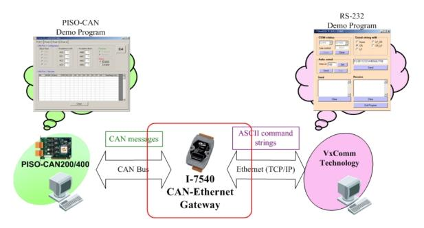
Figure 6-1 Architecture of the demo in PISO-CAN200/400 PCI card
