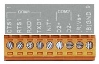
Table 2-1: COM Connector Pin Assignment
