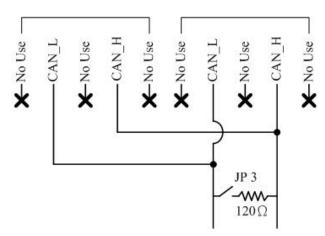
Figure 2-3 Electronic circuit of CAN bus connector
