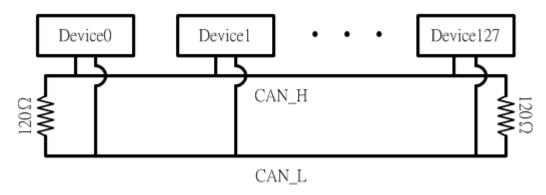
Figure 2-4: Terminator resistor
