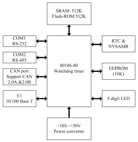
Figure 2-1: Block diagram of I-7540D
