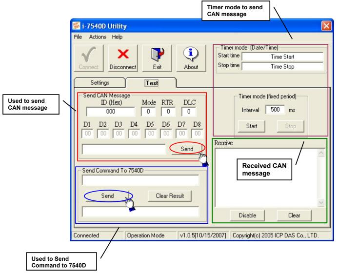
Figure 3-18: Send and receive CAN messages
