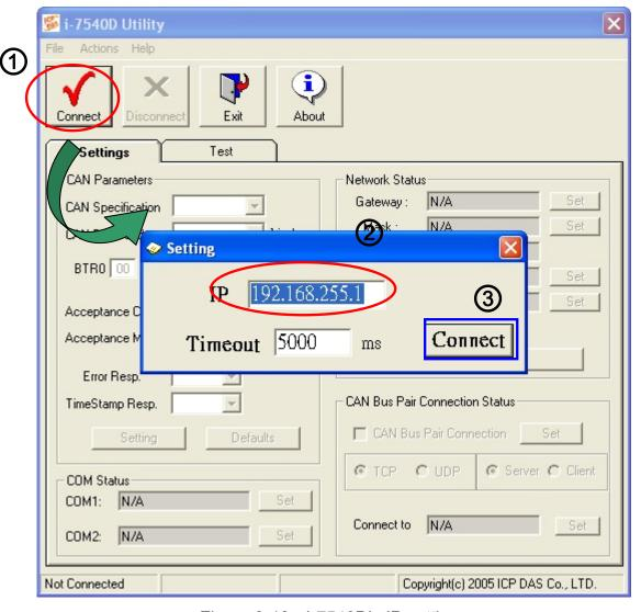
Figure 3-13: I-7540D's IP setting
