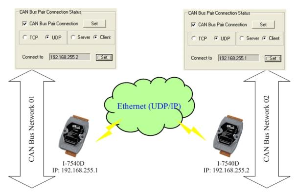
After setting "CAN Bus Pair connection Status" of the two I-7540D and re-start the system of them, CAN messages between "CAN Network 01" and "CAN Network 02" can be exchanged by UDP/IP protocol through Ethernet network.
