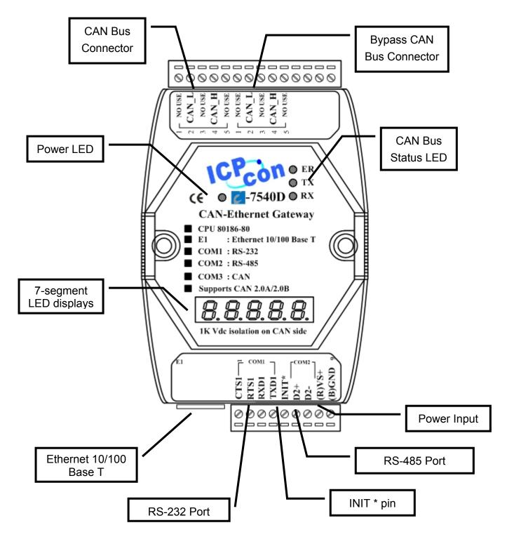
Figure 2-2: Pin assignment on the I-7540D
