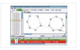
events are updated to the NMS to help users easily maintain the network system. Like as the NMS, not only supports topology discovery, it also delivers group IP assignment, firmware upgrade, configuration files backup / restore,SNMP MIB Broswer /compile, MSR<sup>TM</sup> group management and also allows user to export topology map to drawing file-JPEG, BMP, PNG or PDF for other application.
