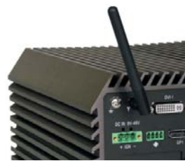
integrated mPCIe module for Wireless Communication (Wi-Fi / 3G / GPS).
