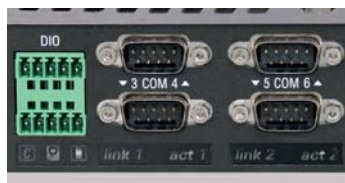
System module with 4 COM & 2 isolated digital I/Os.
