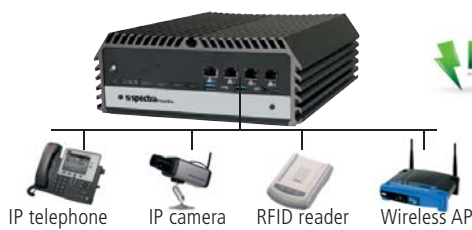
System module with 4 Gigabit-LAN or 4 PoE.
