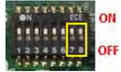
**MODE\_SEL6 / MODE\_SEL7 Pin Defined: COM5 / COM6 Power Select**
