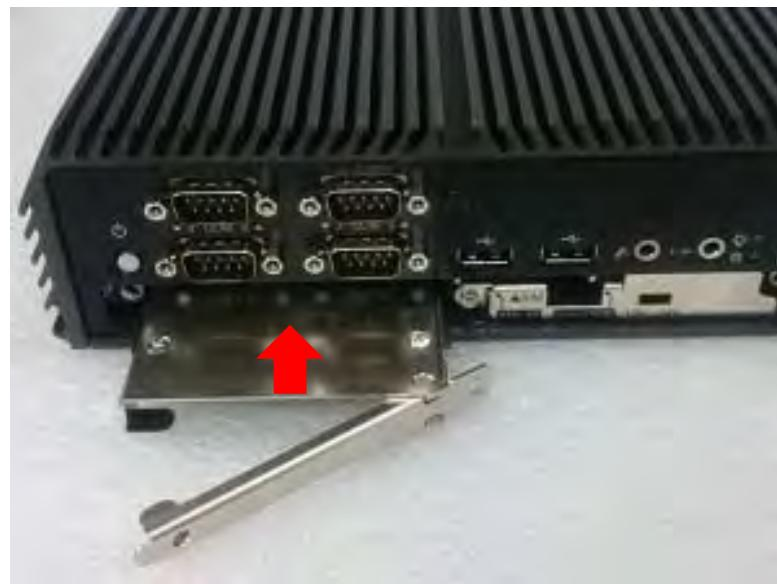
5. Place the rotating arm back and fasten the screw.
