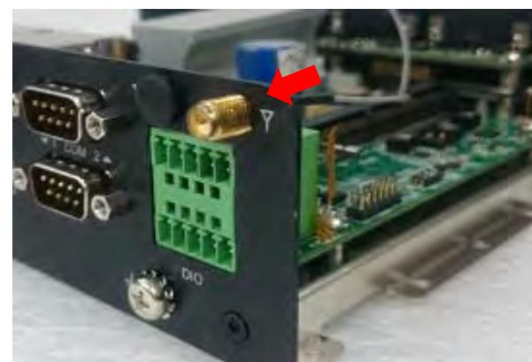
**Caution:** Installing an antenna jack greater than 9mm in diameter at left side of system will be colliding with DIO terminal block connector populated on DIO ports. For the case, please try to install the antenna at left side of system.
