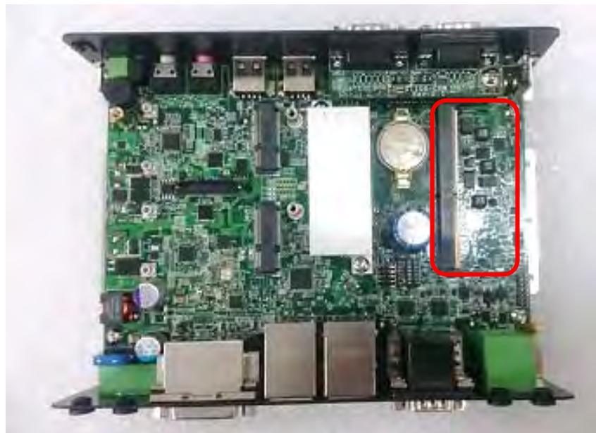
2. Insert a SO-DIMM module at a 45 degree angle until its edge connector is connected to SO-DIMM socket firmly.
