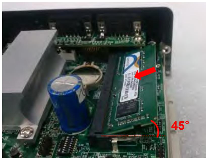
3. Press down the module until the retaining clips snap back in place.
