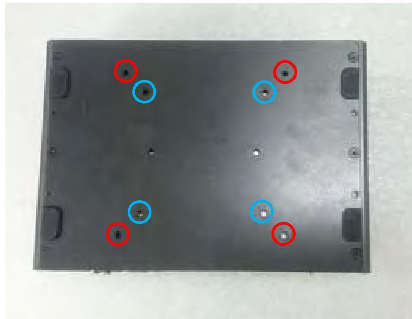
1. The following picture illustrates the installation of Spectra PowerBox 300 series on a VESA stand. Align the 4 screw holes of VESA stand with the screw holes on bottom side of system. Fasten 4 screws to fix it.
