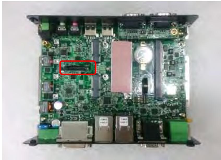
4. Insert the CMI module vertically into the female connector on system's mainboard until it's connected firmly. Fasten 3 screws to fix it.
