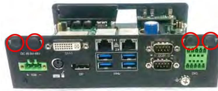
2. Penetrate the antenna jack through the hole at both sides as illustrated.
