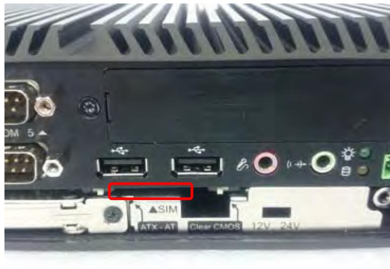
2. Insert a SIM card into the SIM slot.
