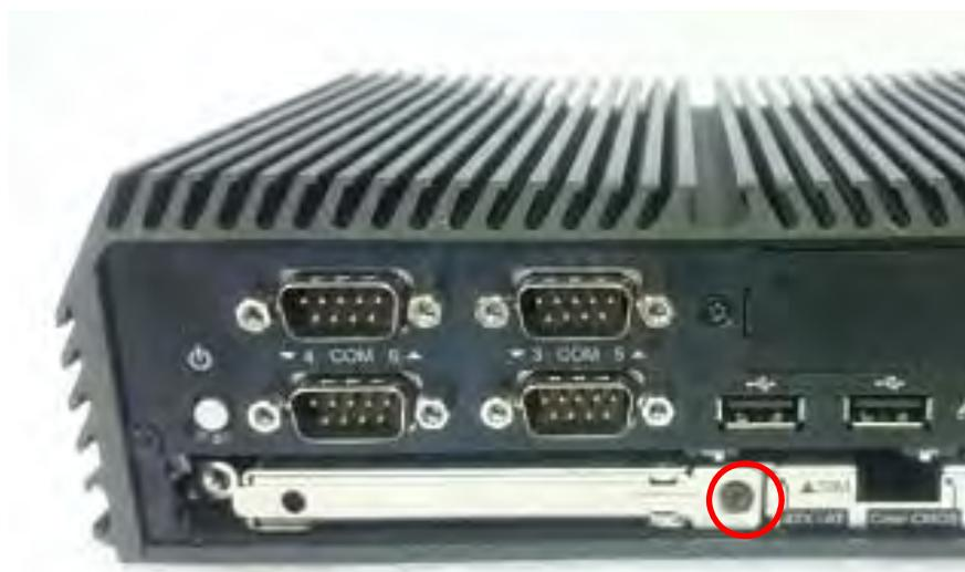
2. Pull the rotating arm and pull the HDD bracket out of system.
