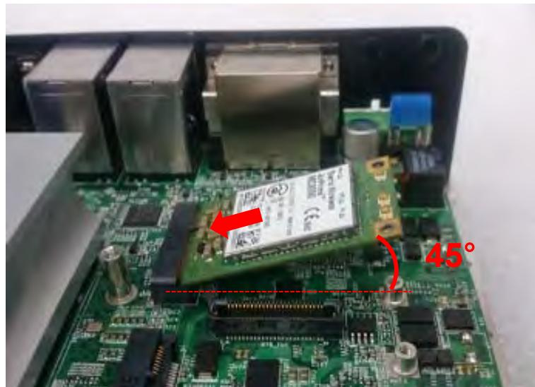
3. Press down the module and fasten two screws to fix it.
