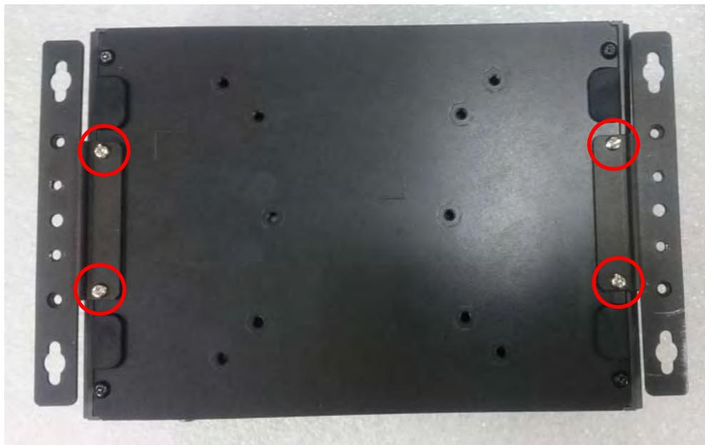
2. Fasten 2 screws through the bracket mounting hole at left and right side to fix the system on the wall.
