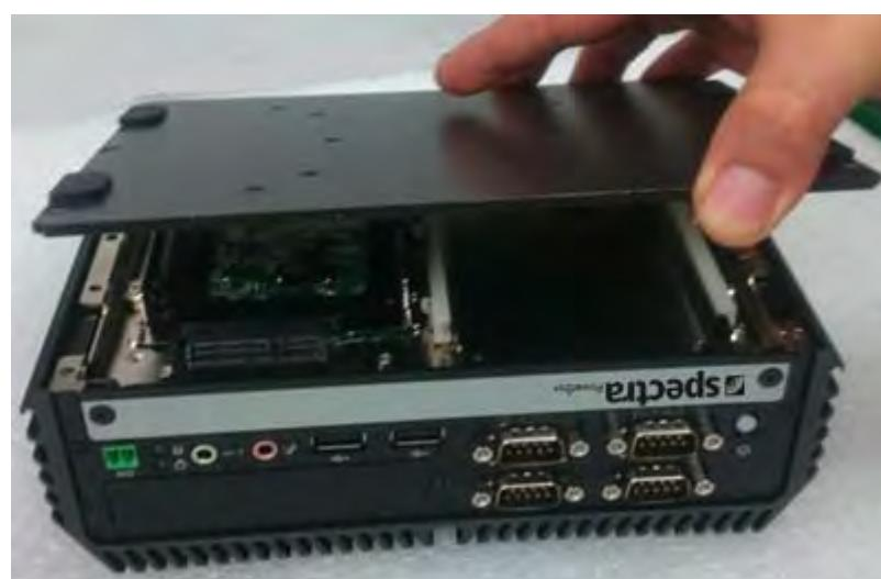
3. Hold front and rear panel and lift up the body of unit vertically.
